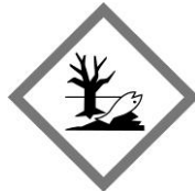
Danger Hazardous to aquatic life
